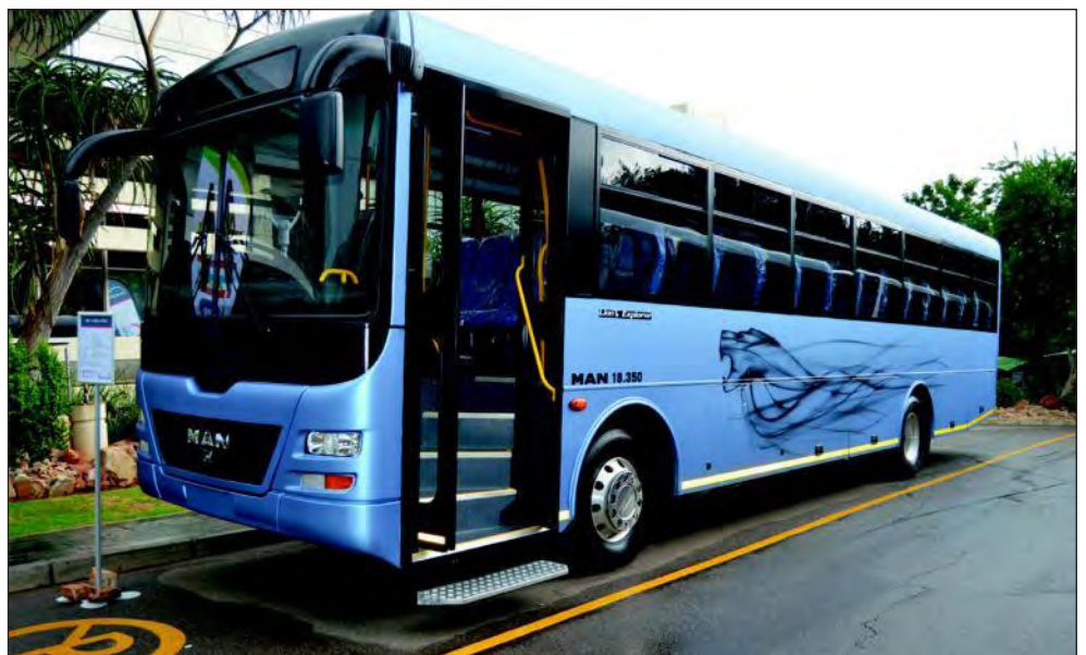
MAN has unveiled its HB3 18.350 FOC Lion's Explorer, combining impressive horsepower with air suspension and TipMatic automated manual transmission.
